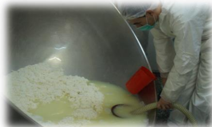
Figure 38 : Separation of cheese from hot water with a pump
