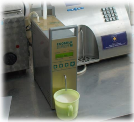
Figure 36 : Analysis of a milk sample (pH, fat, protein, freezing point)
