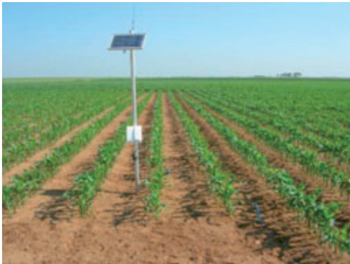
Fig. 1. Sentek probe in a field of corn.
