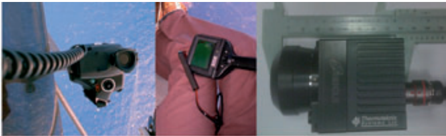
Fig. 8. Examples of thermal camera with remote screen control on ULA - small thermal camera for UAV.
