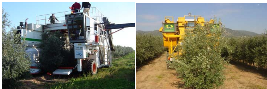
Fig. 10. Straddle harvester for intensive (left) and high-density hedgerow (right) olive orchards.
