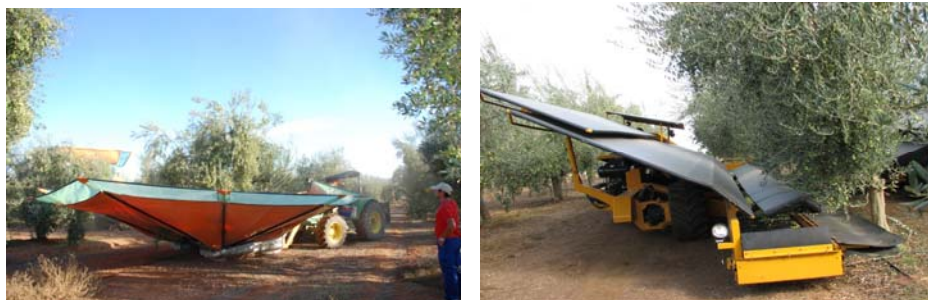
Fig. 9. Inverted umbrella trunk shaker (left) and side by side trunk shaker (right) in intensive olive orchard.
