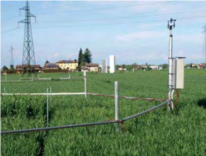
Figure 1. Two of the durum wheat FACE octagons in April 2012 with the CO 2 tank in the background.
