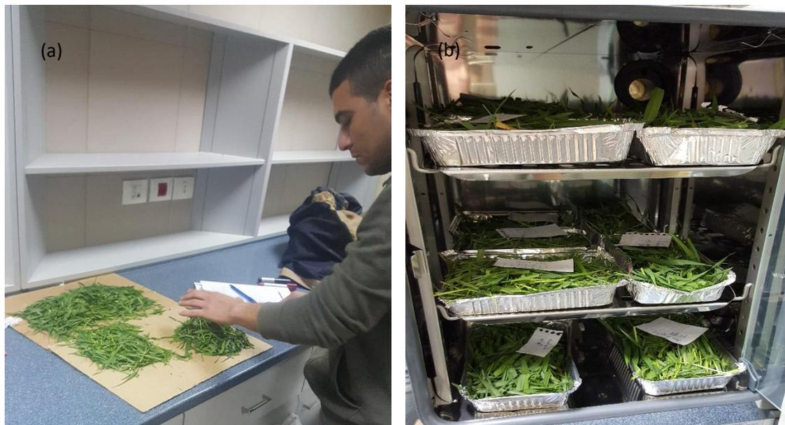
Figure 5 (a) Quartering and (b) biomass samples oven-drying at 70°. Procedure done for all replications in all winter wheat reference plots.
