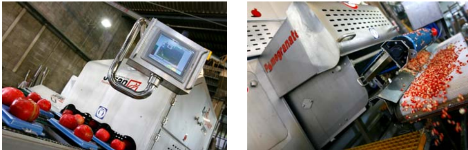
Fig. 2. Arils extraction technology: A patented principle of operation (i) Current Field Capacity: up to 56 fruits per minute; (ii) Operates in 10 countries with over 30 installations.
